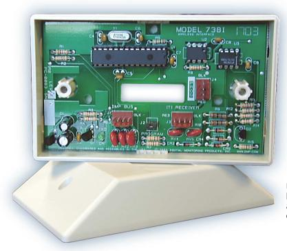
Upgrading to a DMP Command Processor<sup>™</sup> panel has never been easier! The 738I ITI Interface Module allows you to use 96 zones of ITI Wireless equipment on the DMP Command Processor<sup>™</sup> panel.
